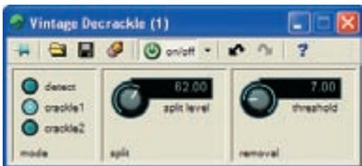
**VINTAGE DECRACKLE** — Uses the same algorithm as the award-winning CR-1 Decrackler. It will also remove some forms of buzz and amplitude distortion from material spanning cylinder recordings to live broadcasts with lighting buzz.
