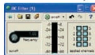
DC removal is normally the first step. Offering 12dB/octave roll-off in the user defined range 1Hz - 20Hz, a display shows the
