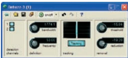
**DEBUZZ-3** — Buzz is defined as unwanted audio with many high-level, closely spaced harmonics. DeBbuzz-3 provides full-bandwidth processing, removing components across the entire audio spectrum, and is capable of removing all manner of buzzes and hums with fundamental frequencies as high as 500Hz. It can also track buzz varying by small percentages. Unlike alternative strategies it retains wanted signal even at the buzz harmonic frequencies by analysing the dynamics of the signal and buzz.
