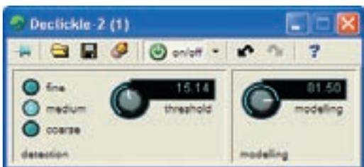
**DECLICKLE-2** — Early digital declickers and decracklers could and did damage the sound of brass instruments, solo violins and sometimes singing. Declickle 2 has an improved noise detector and interpolator and offers improved performance by retaining useful information during clicks and crackles.
