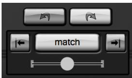
Use the selection tools to define a suitable instance of the unwanted sound and then click on the now illuminated Match button to initiate identification. In the following screen, the darker instance in the centre of the screen is the one selected by the user, and the other grey areas are those identified by Retouch.
