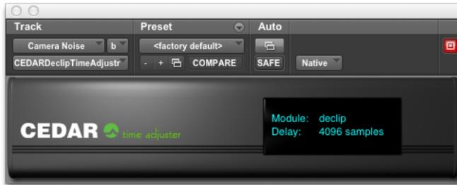
The plug-in delay compensation in some versions of Pro Tools is limited to a maximum of 4,095 samples. However, the propagation delay through Declip is longer than this, which can lead to loss of synchronisation if one or more tracks are passing through the process and others are not.
