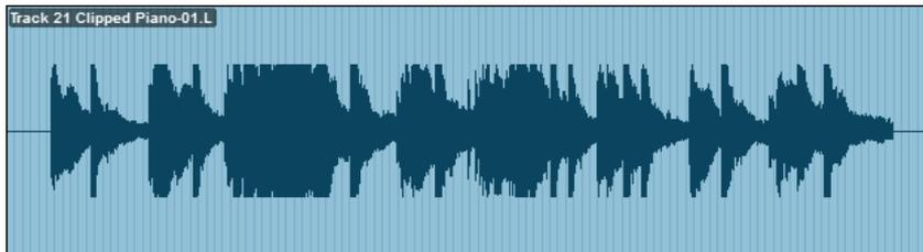
Declip 2 identifies and removes most instances of clipping in a single pass. It does so by presenting a visual indication of the density of sample values in the signal. If the Signal Analysis window displays 'hard' vertical edges it demonstrates that the signal has been clipped at that sample value and that you may use Declip to remove the offending samples and reconstruct the signal.
