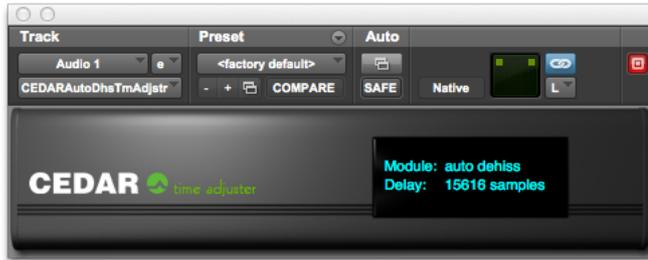
The plug-in delay compensation in some versions of Pro Tools is limited to a maximum of 4,095 samples. However, the propagation delay through Auto Dehiss is longer than this, which can lead to loss of synchronisation if one or more tracks are passing through the process, and others are not.
