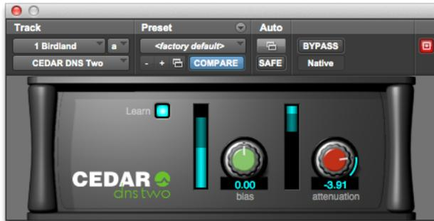
DNS Two is a further development of our DNS technology. It dispenses with the manual control offered by DNS One's range selectors and band gain controls and uses an enhanced Learn function to analyse the noise and then calculates the internal parameters necessary to suppress it. DNS Two is not a cut-down version of DNS One; you will find many cases in which it's not only quicker and simpler to use, but will obtain superior results to DNS One.
