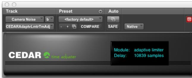
The plug-in delay compensation in some versions of Pro Tools is limited to a maximum of 4,095 samples. However, the propagation delay through Adaptive Limiter 2 is longer than this, which can lead to loss of synchronisation if one or more tracks are passing through the process, and others are not.
