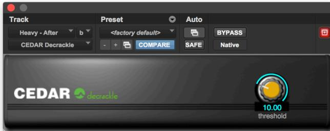
Decrackle is based on a process invented by CEDAR called 'Split & Recombine'. It removes surface noise, crackles, and some types of buzz. You may also use it to reduce the audible effects of some amplitude distortions.
