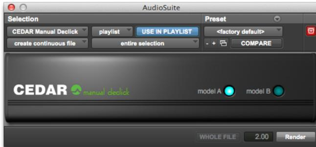
Manual declick should be used to remove extended clicks. It allows you to specify the audio that constitutes the click and restores the audio using an interpolator that is optimised for longer clicks and scratches. The maximum click length handled is approximately 0.1s irrespective of sample rate.
