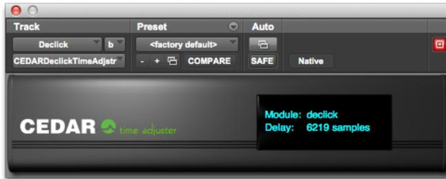
The plug-in delay compensation in some versions of Pro Tools is limited to a maximum of 4,095 samples. However, the propagation delay through Declick is longer than this, which can lead to loss of synchronisation if one or more tracks are passing through the process and others are not.
