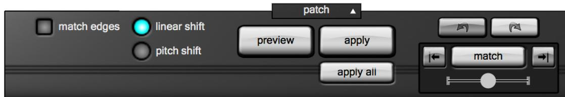
To replace an unwanted burst of noise with some audio from nearby, select Patch mode and define the region that you are going to patch. No wings will appear because they are not appropriate for this operation.
