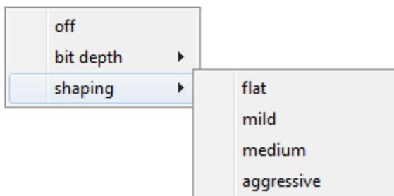
Audio may be dithered and, if desired, noise-shaped, by selecting one of the four options. Choose 'flat' for TPDF dithering, or one of the three forms of noise shaping as desired.
