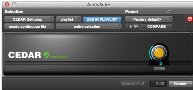
Dethump should be used to remove low frequency disturbances. The maximum thump length handled is approximately 1s irrespective of sample rate.
