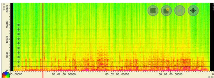
Invoked within the spectrogram menu, harmonic markers allow you to view the first ten harmonics of a given fundamental frequency. Drag any of the markers to adjust the fundamental and, therefore, the other nine harmonics. Markers can be very useful when, for example, identifying the harmonics of a tone that you wish to remove or shift in frequency to correct a wrongly played note.
