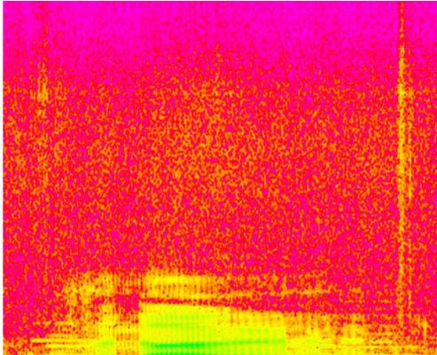
Select an appropriate value for Synthesis. In this example, the maximum value of 100 is correct because (i) there is no obvious meaningful signal within the marked region, and (ii) the audio adjacent to the marked region appears to be consistent and therefore a good model for the replacement.
