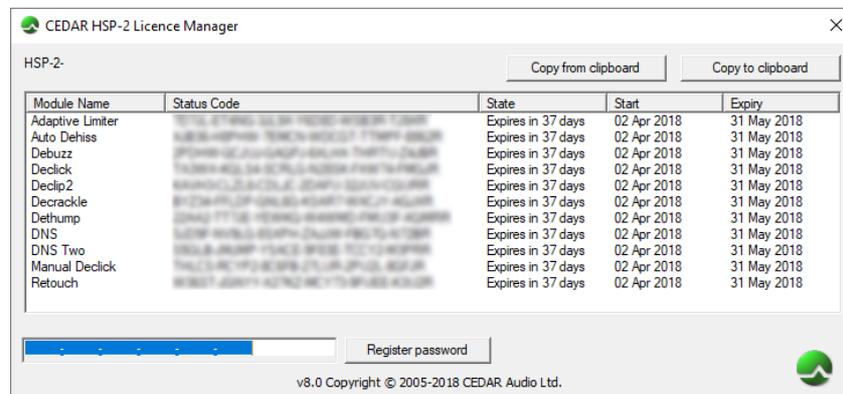
To install a licence that connects new software to the existing dongle, type the password supplied by CEDAR Audio into the **Register password** window. (You may also **Copy from clipboard** if appropriate.) When accepted, the password will change from red to black. Press the **Register password** button to complete the registration. The new software is now ready for use.
