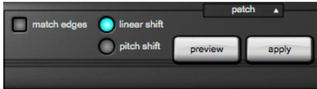
To replace an unwanted burst of noise with some audio from nearby, select Patch mode and define the region that you are going to patch. No wings will appear because they are not appropriate for this operation.
