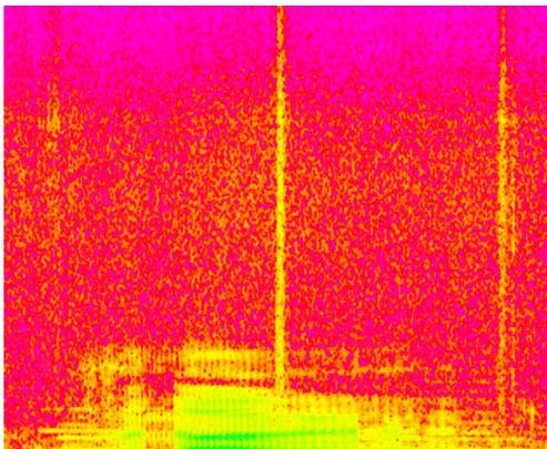
This spectrogram shows about two seconds of 44.1kHz audio. You can see two yellow vertical bars that represent two loud events, one in the centre, and one to the far right. We will concentrate on removing the one in the centre.
