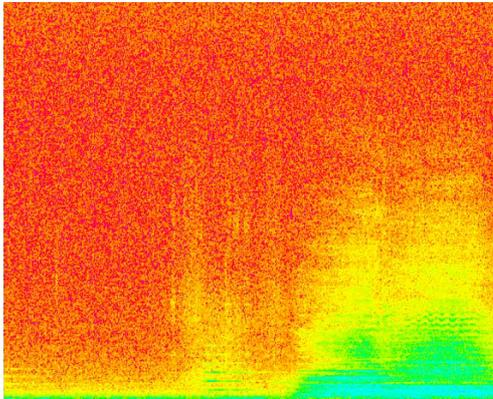
This spectrogram shows the sound of a car horn that occurred during a piece of otherwise wanted signal. You can see this as a small region of green horizontal lines in the centre/bottom of the display.
