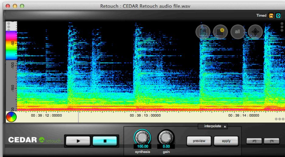
To maximise the resolution on the colour axis, it is useful to fit the entire range of the colour wheel within the highest and lowest amplitudes in the Retouch window. Furthermore, it is often useful to represent low amplitudes as black areas on the spectrogram, and high amplitudes in white. You may make these adjustments (which can be thought of as zooming on the Z axis) using the Amplitude Bounds controls and menu.
