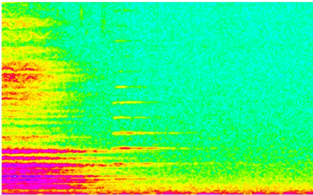
Having identified the harmonics by eye, mark them as shown using the Add to Existing Selection tool or by pressing <SHIFT> while marking them individually.
