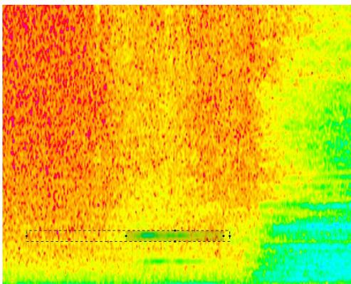
There is nothing to stop you from processing the unwanted noise in one application of Retouch, mapping out the whole area in a single sweep of the Interpolate tool, but you will achieve better results if you apply the process individually to each harmonic. This is because, if you mark the whole region as unwanted, you will be including much of the breath sound as 'bad', when it clearly is not. A more precise approach ensures that you remove the bad sound with minimum impact upon the good.
