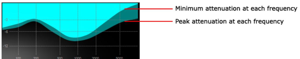
The action of the Adaptive Limiter is shown by the two lines in the display.
