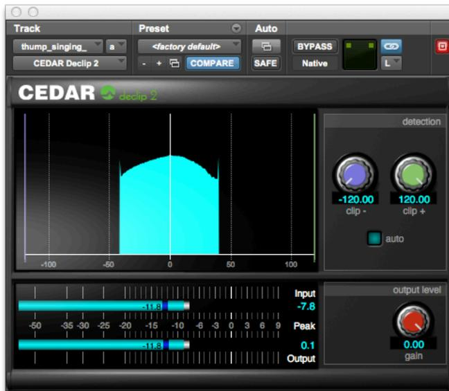
Clipping occurs when a piece of equipment or a medium carrying a signal is unable to handle a high level presented at its input, and will usually be heard as a harsh distortion that increases in intensity as the clipping becomes heavier. In all cases of clipping, it is the portions of the waveform near its extremities that are affected, while portions of the waveform closer to zero are unaffected.
