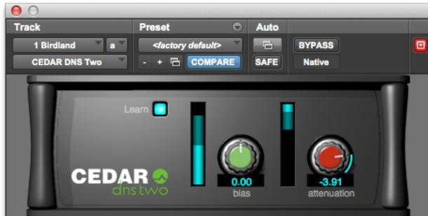
DNS Two is a further development of our DNS technology. It dispenses with the manual control offered by DNS One's range selectors and band gain controls and uses an enhanced Learn function to analyse the noise and then calculates the internal parameters necessary to suppress it. DNS Two is not a cut-down version of DNS One; you will find many cases in which it's not only quicker and simpler to use, but will obtain superior results to DNS One.
