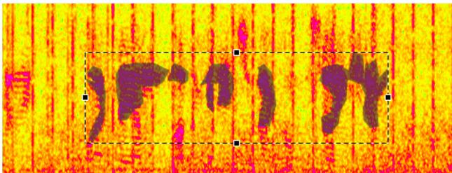
Now choose appropriate value for the Inner (marked) and Outer (unmarked) volumes. In this example, we have left the amplitude of the wanted sounds unaffected but attenuated the background by 50dB.
