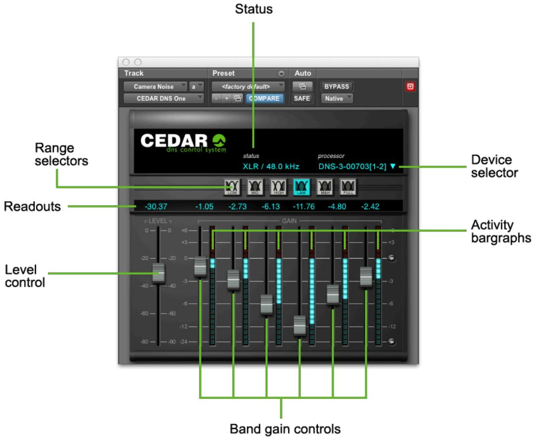
You can connect Pro Tools to the CEDAR DNS2000 and DNS3000 dialogue noise suppressors using the DNS CS control system.
