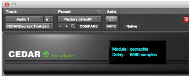
The plug-in delay compensation in some versions of Pro Tools is limited to a maximum of 4,095 samples. However, the propagation delay through Decrackle at high sample rates is longer than this, which can lead to loss of synchronisation if one or more tracks are passing through the process and others are not.
