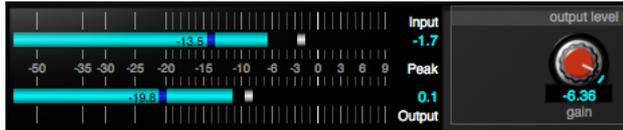
The peak amplitude of a declipped signal can be significantly greater than that of the incoming signal. To output this without reintroducing clipping, it may be necessary to attenuate the signal. Use the Output Gain control to fit the restored signal into the available headroom.
