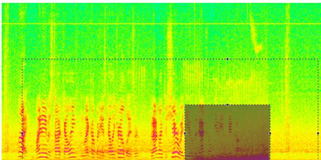
A large area has been marked around the region containing the roar. Retouch uses the information in this to build a model of 'good' audio which will be used to retain those elements in the marked region that are also deemed to be good, while attenuating those that are not.
