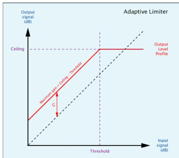
This above illustrates the relationship between the input signal level and the output signal level, and shows how this is affected by the Threshold and Ceiling controls. These can be defined as follows:
